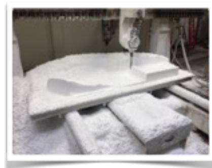
*The CNC Machine carving the wave; Photo Credit: Kelly Hand, Satellite Models*
